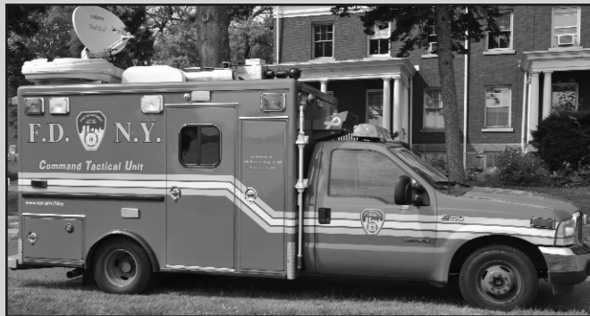
The CTU is a refitted ambulance that provides vital information to the IC by using cameras, a network system and satellite dish.
